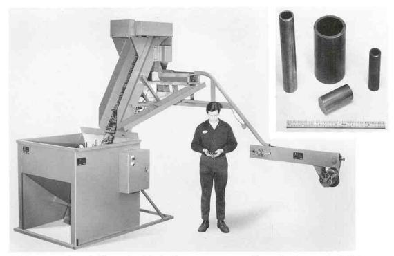
This feeder gets a host of different pins, shafts, bushings and pistons (9/16 to 2 inches diameter by 1-3/4 to 6-1/2 inches long) to our customer's centerless grinder.
