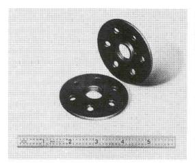
Mounting plates for spin-on oil filters are fed to six tapping spindles at more than 90 pieces per minute,
