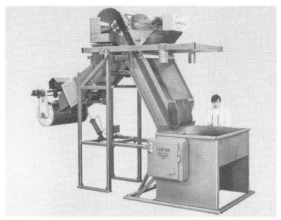
This Spectrum storage feeder uses a batch weight discharge unit to get parts into chemical treatment carrier baskets.
