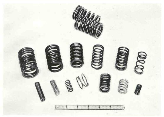
Springs, like these, are handled best with Spectrum's orienting, separating, inspecting and distribution methods. Close wound ends can be end selected
