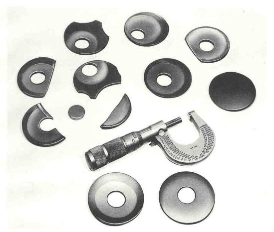
We use common sense methods to sort and feed these retainer washers at 125 pieces per minute, Even the hole is probed for location.
