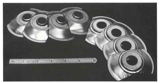
Here are two kinds of sheet metal springs for automotive oil filters. We feed them at 60 pieces, per minute, for assembly purposes.
