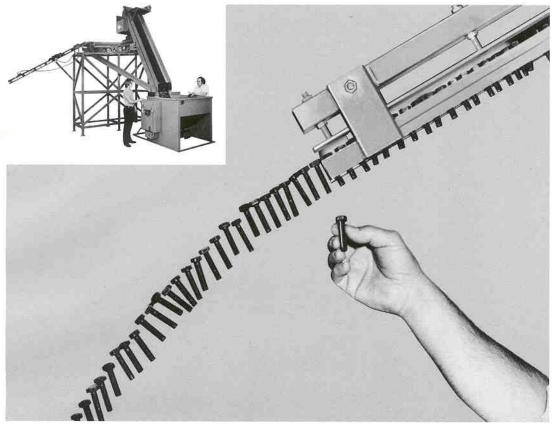
This machine delivers bolts and screws to: threadrollers; burnishers; trimmers; pointers; and other fastener making machines. It will orient and feed 1/4 to 5/8 inch diameter parts to 6 inches long.
