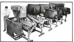
These ball joint parts are live fed, direct to the fixtures of an automatic assembly machine. No troublesome gravity track.
