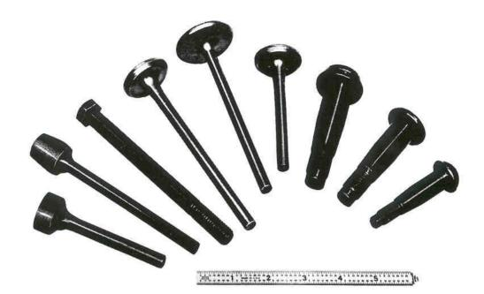
Screws, bolts, rivets and the like are fed near 400 per minute (up to 1½ inches long). Longer parts are fed somewhat slower. Engine valves are fed at 100 per minute with a noise limit of 80 dBa.
