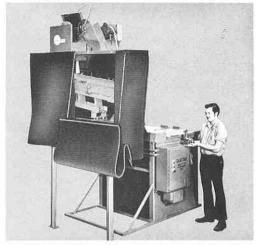
Simple, quickly adjusted, orientor tooling sorts out largest part at 350 per minute while the smallest race is tramp materials and feeds this family of bearing races for process, assembly or packaging operations. Changeover from part to part takes less than twelve minutes.
