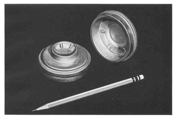
These servo pistons are stored in a 12 cu. ft. bin, elevated, oriented, distributed to two paths and tracked to a pair of chuckers.
