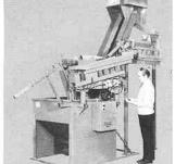
This feeder assembles a family of bolt blanks to flat or concave washers, from bulk, through amazingly simple tooling. No mechanical functions are used.
