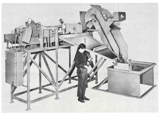
This Spectrum extra heavy duty storage feeder gets automotive front suspension cross shafts onto a washer-furnace conveyor. Two kinds of sixteen inch shafts are oriented and then escaped in rows of four at 44 per minute. They are released through stagger chutes because four, end
