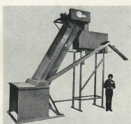
A variety of steel billets; 7/8'' to 2-3/8'' diameter by 7/8'' to 3-1/2'' long, are fed to an induction heater for hot forging into socket wrench blanks.
