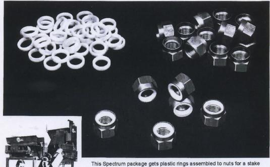
This Spectrum package gets plastic rings assembled to nuts for a stake operation at more than 175 pieces per minute.
