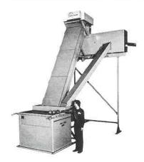
Rotor segments are stored, elevated, oriented and fed to an assembly operation.
