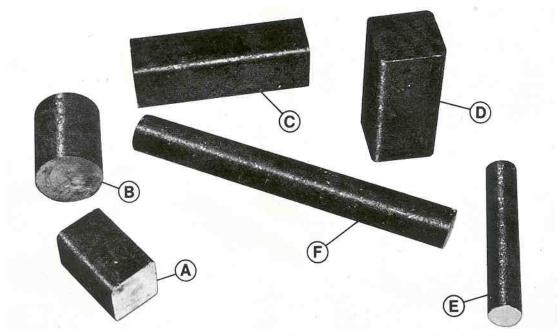
These steel billets are delivered to the load chute of an induction heater at 400 pieces per hour. The feed system includes a stock box dumper, floor bin and elevator, orientor, feed track and escapement.
