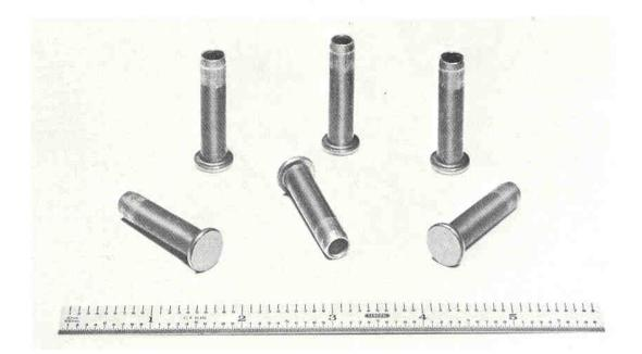
These rivets are stored, elevated, oriented, escaped and blown through a plastic tube to an assembly station from a remote location.
