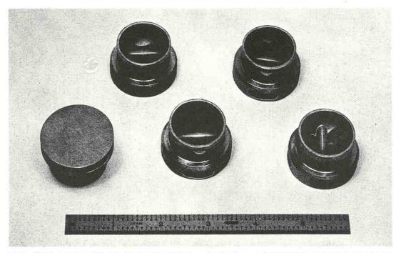
These diesel engine parts are fed to a centerless grinder at 60 pieces per minute. They are stored, elevated, oriented, tracked and escaped onto a feed conveyor.
