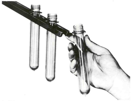
This SPECTRUM feeder stores, elevates, orients and feeds a range of PET preform sizes at better than sixty pieces per minute.
