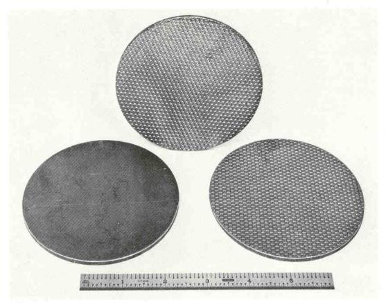
Two feeders are used to get these embossed (one face) blanks into twin nests of a press feed dial.
