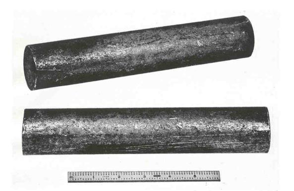
These nine pound steel billets are stored, elevated, oriented, inspected for length, tracked, distributed and escaped to induction heaters at 840 pieces per hour.
