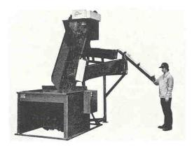
This family of valve stems is stored, elevated, oriented and tracked to an assembly machine at 60 pieces per minute.
