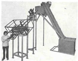
This family of Transmission Valve Sleeves is stored, elevated, preoriented, tracked, end selected, distributed to four paths, identification stamped and presented for automatic processing at 120 pieces, per minute.
