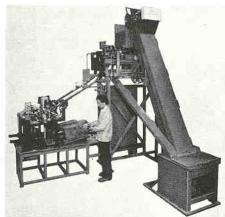
Lash adjuster bodies are stored, elevated, oriented and fed to the magazines of two ball seat polishing spindles at 120 pieces, per minute.
