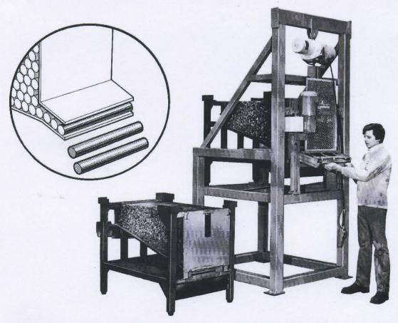
This unique rod feeder concept can be adapted to one or a family of diameters and lengths.
