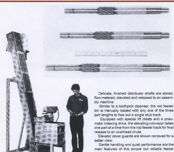
flow metered, elevated and released to an assem-
