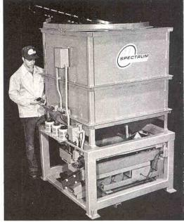
Tracked to a Spectrum Gentle Bin storage unit, these finished planet pinion gears are lowered, by internal track, and gently accumulated to 20,000 pieces in random bulk.
