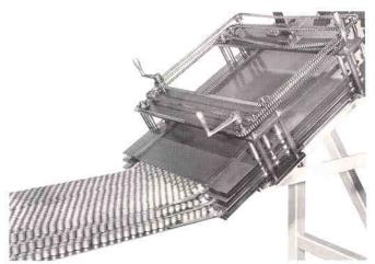
Fifteen different parts, like these, are stored, elevated, oriented, distributed to three paths and flow metered onto a heat treat furnace belt at 150 to 300 pcs. per minute.
