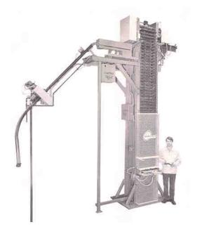
Bulk handling is commonplace for auto-feeding ball studs and tie rod ends *before* they are assembled.
