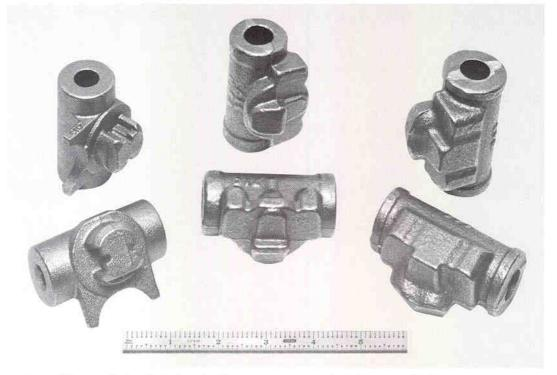
Four different Brake Cylinder Castings are dumped, stored, elevated, oriented, live feed tracked, and presented for robotic pickoff at eight pieces per minute.
