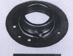
This hat shaped metal stamping is bulk stored, flow metered, oriented, and live fed to a process operation at 70 pieces per minute.
