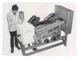
A Nut and two Ferrules are auto fed and assembled at 45+ cycles per minute by three Spectrum straightline (non-bowl) vibratory feeders.
