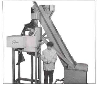
Bowl feeders were purchased to handle this window crank assembly. It has an internal coil spring topped with grease. Results: grease lined bowls and **unreliable** performance.
