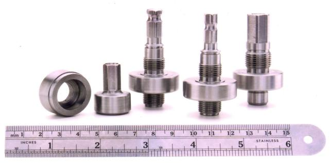
This feeder has full menu of designed, quick-change, bolt-in tooling for eight different Arbors and Caps.
