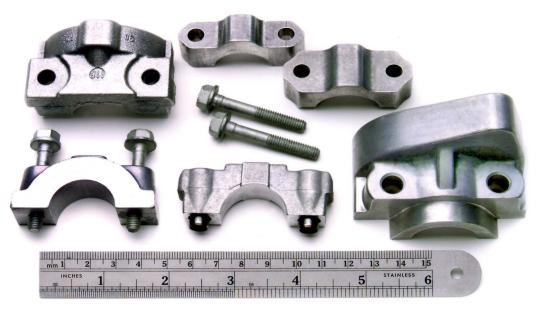
This is a sample variety of Cam Shaft Bearing Caps that have been fed with many Spectrum gentle handling concepts. Caps, some with dowels, are stored, elevated, and oriented (some via multi-path).
