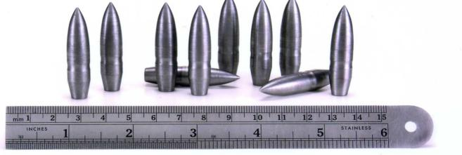
50 Calibre Projectiles are gently fed at 30+parts per minute for tracer treatment. A one cubic foot storage bin with and clevating conveyor gently delivers parts to straightline vibratory drives for orientation and live feed tracking.
