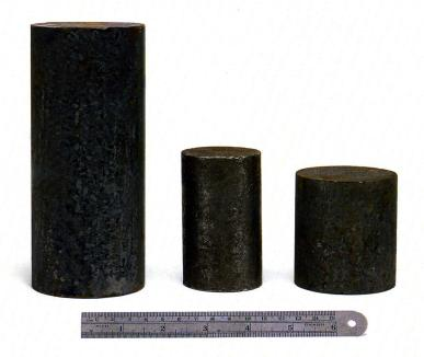
like these, are fed to an induction heater at 15 to 35 pieces per minute at an average noise of 85 dB(A). Parts are dumped from a stock box into a floorbin, then elevated to an orienting conveyor to exit, end to end, via a short track.
