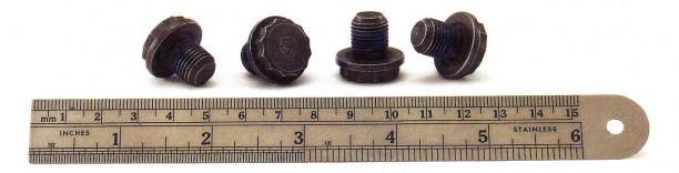
Flex Plate Bolts are bulk stored, elevated, vibratorally oriented, live fed and escaped to a pick-and-place unit. A rotary indexer, with seven position bolt tooling plate is loaded by the pick-and-place every 20 seconds.
