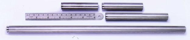
...these steel Tubes (18.5mm diameter X 75-140mm long; one length at-a-time) are fed to an end cap weld operation.
