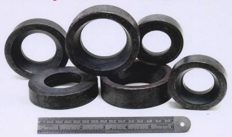
A family of twenty six RINGS (67 to 91mm O.D. x 18 to 35mm thick) is fed, one size at a time, through an induction heater to a forge operation.
