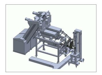
Floorbin elevators are used to store, elevate, and bulk feed a wide variety of parts, over-the-top, to various overhead chutes and manipulators. In this system designed for a customer in the automotive industry, two different part variants are loaded into the hoppers. The parts are lifted through the hopper elevators. Parts are dropped down the in-feed chute, into the vibratory orientor.
